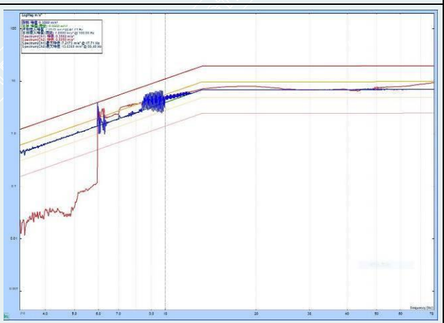
Fig.5-4 Resonance point search curve (X)
