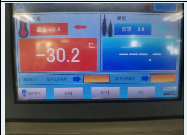
Fig.3-4 Temperature interface (low temperature storage)
