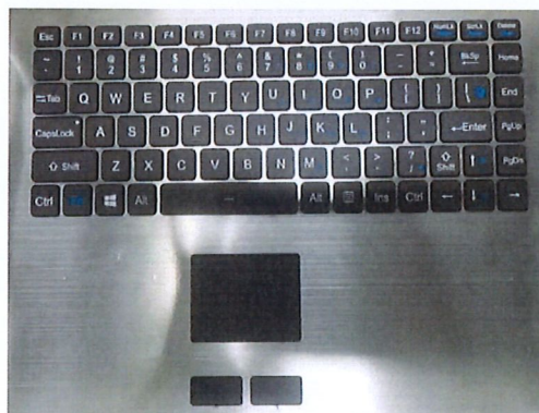
Fig.1 Waterproof Scissor Switch Keyboard
