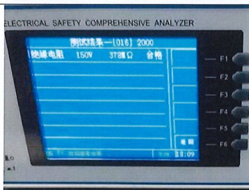
Fig. 6 Insulation Resistance Test (S03)
