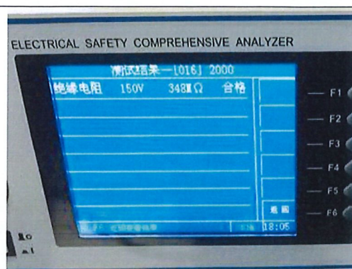
Fig. 4 Insulation Resistance Test (S02)
