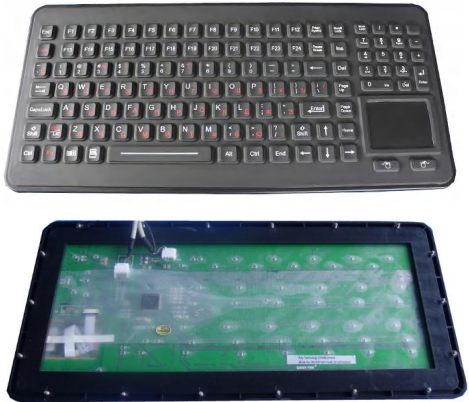
ABS frame with stainless steel bolts K-TEK-M379TP-KP-FN-IL
